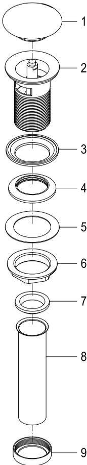
1. Remove parts (4)/ (5)/ (6)/ (7)/ (8) (9) from the drain body (2).
